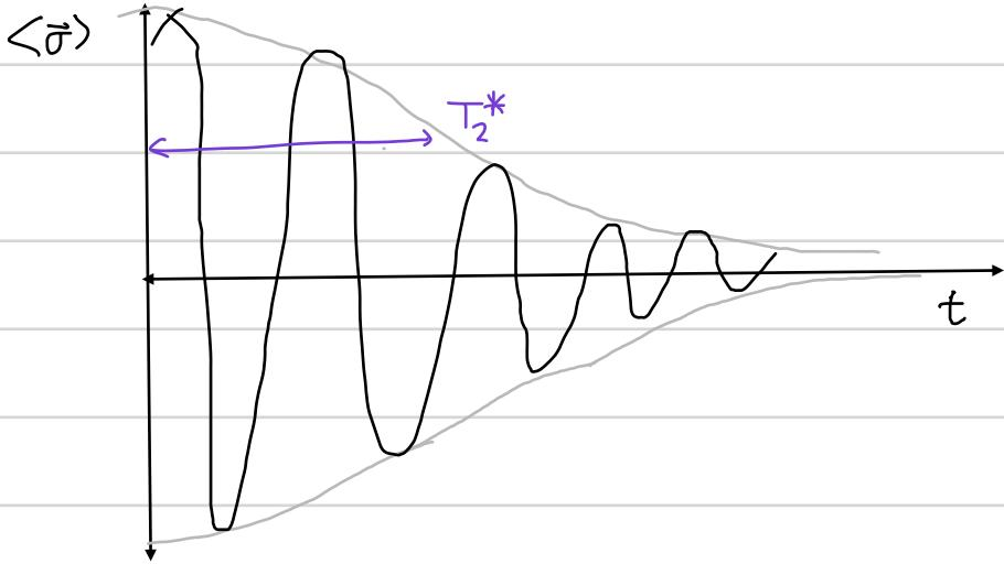
Wave train with a decaying Gaussian envelope due to inhomogeneity.
