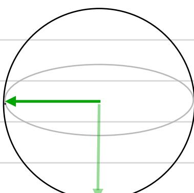
A hard  $\frac{\pi}{2}x$  pulse rotates to  $y$ -axis
