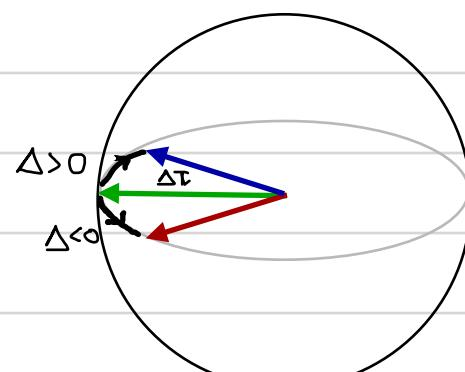
Spins freely precess spread out due to inhomogeneous detunings
